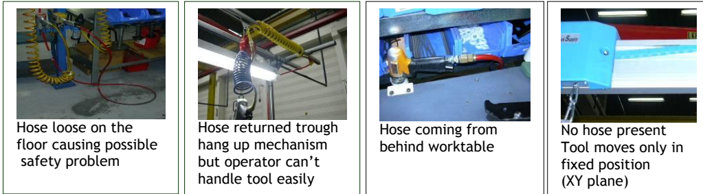
Loose position Figure 2: 5S law on position & controllability applied to a hose and powertool
