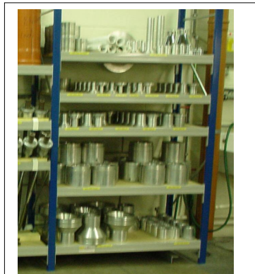
All fixtures are identified and labeled in rack and easily found: Sorted, Straightend and Shining Picture 6
